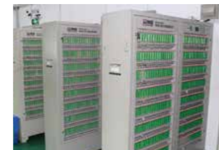
Battery Capacity Detection Cabinet
