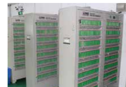
Battery Capacity Detection Cabinet
